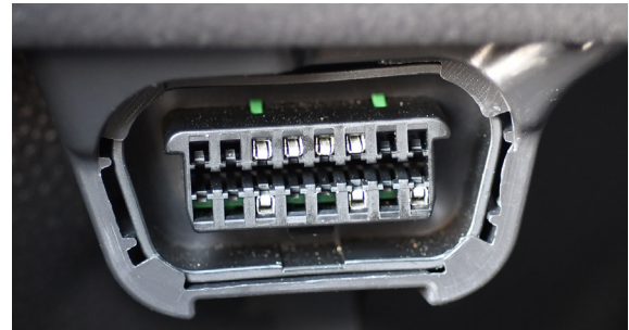
Figure 50: Locate your vehicle's On-Board Diagnostic (OBD) connector. Connect the Stalker CAN/VSS cable.
